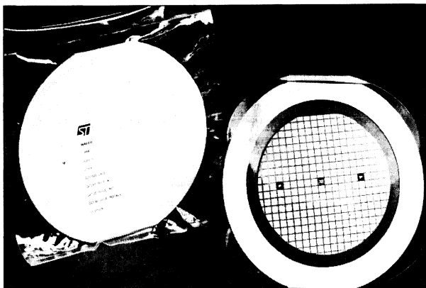
Circle pack Suffix D4: wafer tested inked and scribed at 100%
